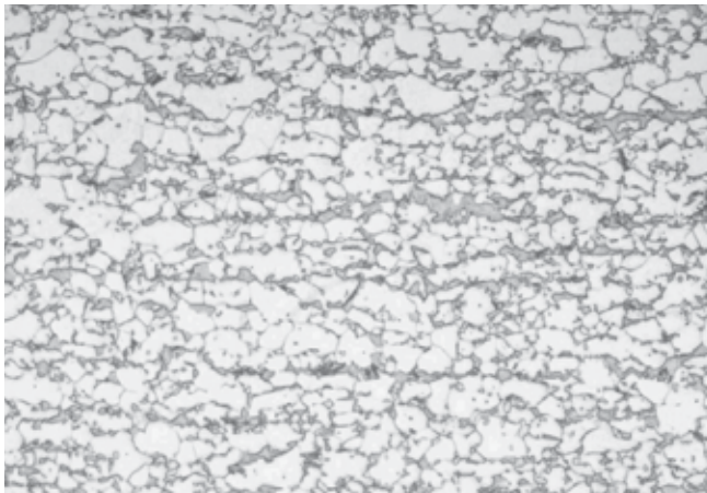
Structural example of cold-rolled DP steels. Microstructural contrasting through etching with nital.
