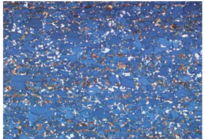
Structural example of cold-rolled DP steels. Microstructural contrasting with color etching according to Klemm.
