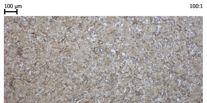
Microstructure consisting of 100% martensite.
