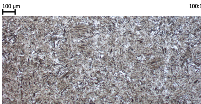
Microstructure consisting of 100% martensite.
